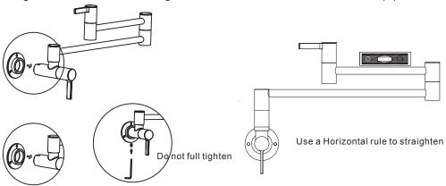
Disassemble the pot filler from the finish wall and drill suitable holes according
