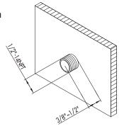
Place Mounting bracket (16) onto pot filler(1); Mount pot filler onto nipple on the finished wall surface, do not full tighten the body to the wall and mark three fixing holes. Ensure that fixing holes will be free from all concealed pip work.
