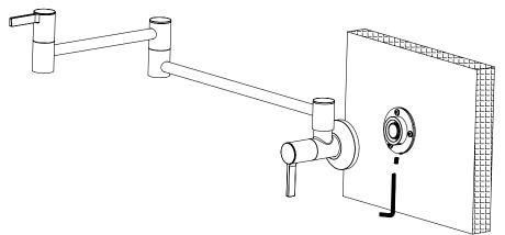
After installation, remove the aerator and turn on the water to remove only debris in the piping. Re-assemble aerator. This tap is equipped with two shut off valves, the wall valve should be closed (handle in vertical position) when faucet is not in use. If the pot filler is to be left unattended, please ensure both valves are left in closed position.
