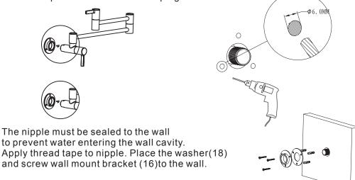
Note: The mounting bracket must be fully attached to the finish wall.
